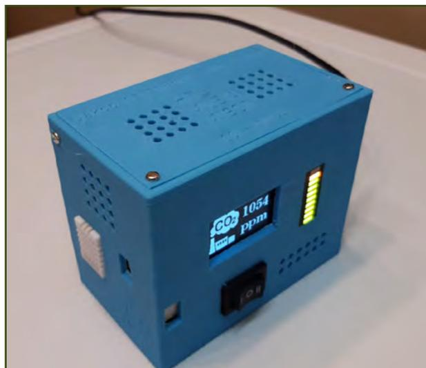
Die CO<sub>2</sub>-Ampel mit Sensoren
